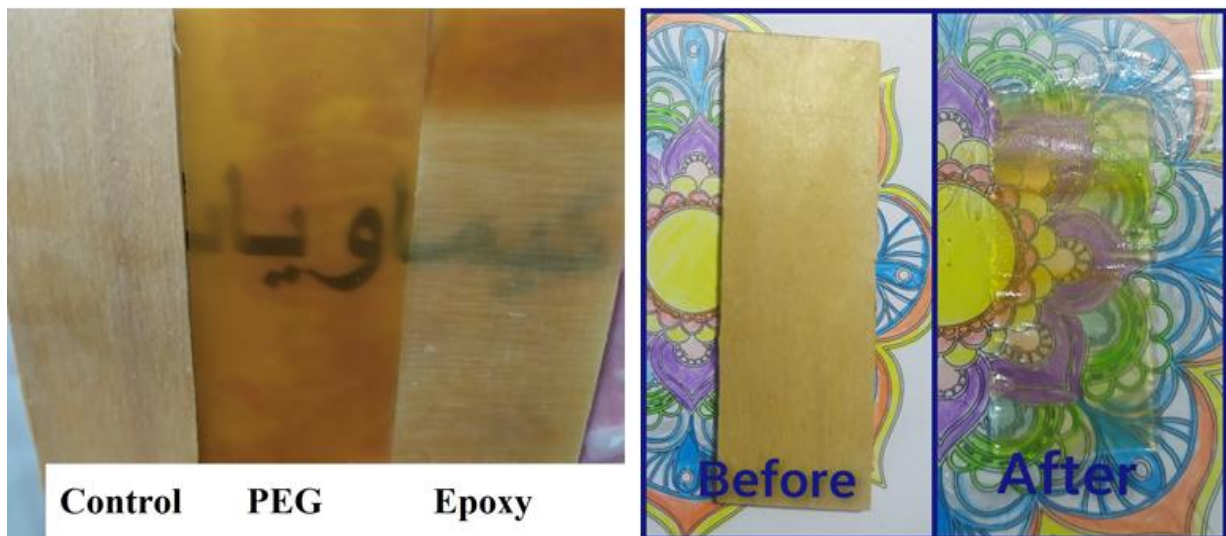
Fig. (3) Wood transparency before and after lignin removal
